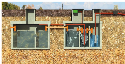
Solution B: Install Treatment Tank Upgrade
